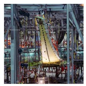
This photo shows Boeing bending a wing on test way beyond anything likely in flight, then
